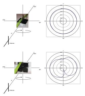
Figure 6: Polar Plots of an Antenna Radiation Pattern
