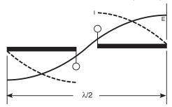
Figure 1: A Half-Wave Dipole Antenna
