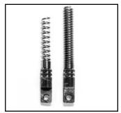
Figure 3: 916MHz (L) and 315MHz (R) Helical Antennas
