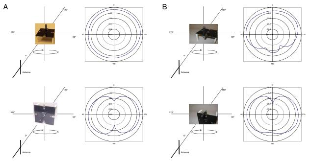
Figure 11: A 418MHz Antenna Radiation Pattern on a 4" x 4" Ground Plane (A) Centered, (B) Edge Mounted
