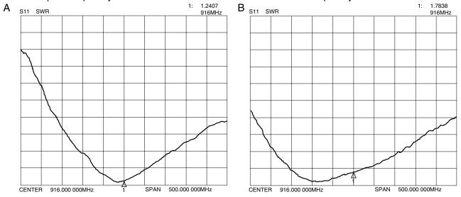
Figure 10: A 916MHz Antenna VSWR on (A) a 4" x 4" Ground Plane and (B) a 26.5" x 26.5" Ground Plane
