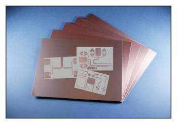
RT/duroid<sup>®</sup> 6006/6010LM microwave laminates are ceramic-PTFE composites designed for electronic and microwave circuit applications requiring a high dielectric constant. RT/duroid 6006 laminate is available with a dielectric constant value of 6.15 and RT/duroid 6010LM laminate has a dielectric constant of 10.2.
