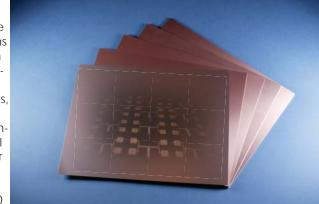
ers need. The laminates have a dielectric constant (Dk) ranging from 3.3 to 3.5 ( $\pm 0.08$ ) and a loss tangent (Df) of 0.0020 to 0.0037 measured at 2.5 GHz. These values allow antenna designers to realize substantial gain values while minimizing signal loss. Materials are available with demonstrated low PIM performance, with values better than -155 dBC using two 43 dBm swept tones at 1900 MHz.
