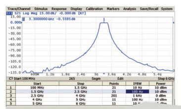
The VNA has a large frequency range with the option of frequency scan segmentation. This allows optimal use of the device, for example, to realize the maximum dynamic range while maintaining high measurement speed.
