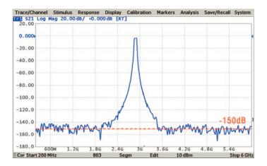
Typical dynamic range of 150 dB is achieved through the entire frequency range (at 1 Hz IF bandwidth). Seen here is the maximum dynamic range achieved when using IFBW 1 Hz and an output power level of 10 dBm.
