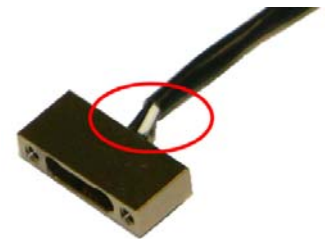
Figure 2. Connector showing wire-pin transition (circled).
