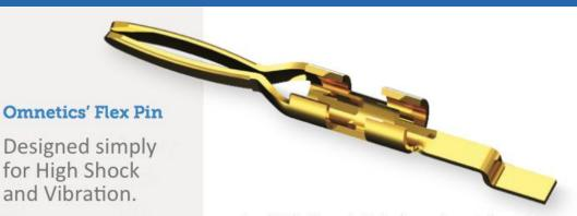
Omnetics' Flex Pin contact design is an engineered piece, designed and produced many years before the creation of MIL-DTL-32139. This simple one piece designis stamped from ASTM B194 BeCu.
