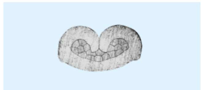
The F crimp results in a well-defined, clean pinch.
