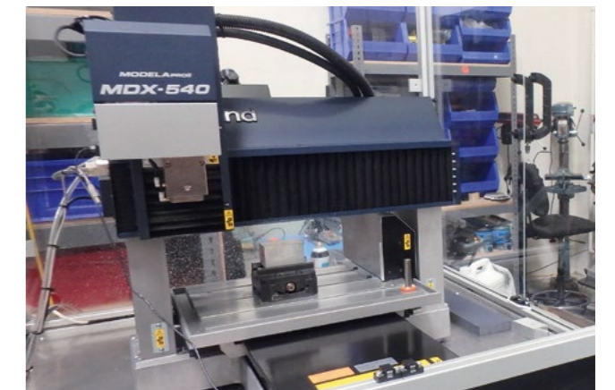
Here we show our milling unit, which is used to produce prototype tools and moulds for customer-specific applications. The simple configuration allows rapid implementation of small series with up to 2,000 units.
