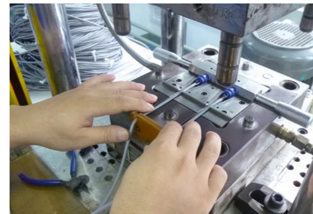
Extrusion of assembled ODU MEDI-SNAP connectors in a master mould with modular interchangeable inserts. Here it is possible to react quickly and flexibly to the widest range of cable diameters that maintain a stable manufacturing process.
