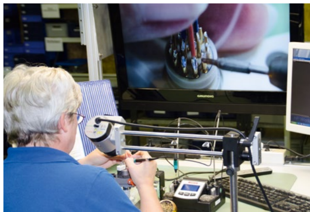
Assembling a patient cable set that documents all solder points by using a camera system. The complete data set is then given to the end customer along with the cable.
