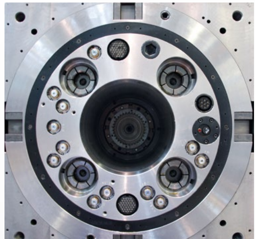
ODU DOCK FOR MILLING AND GRINDING MACHINES (Source: Waldrich Siegen Werkzeugmaschinen GmbH)
