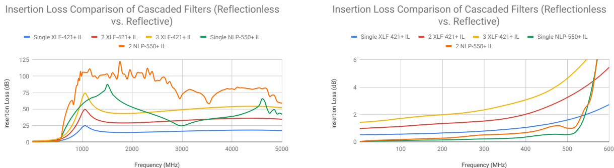
Figure 7: Cascading conventional filters increases ripple in the stop-band and passband. Reflectionless filters eliminated this unwanted effect but introduce an expected accumulation of insertion loss.
