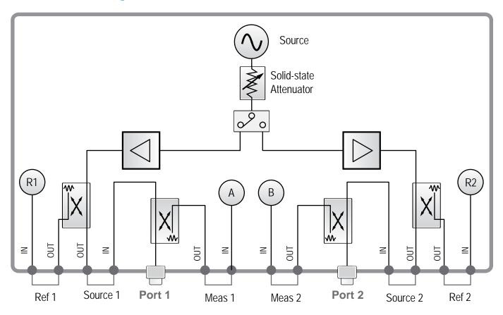
This 2-port analyzer offers adjustable port configuration with direct access to the receivers.
