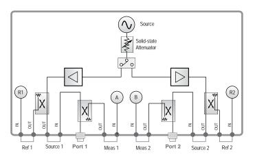
This adjustable port configuration with direct access to the receivers of the VNA provides for a variety of test applications requiring wider dynamic and power range.
