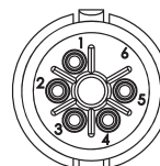
5 POSITION B-KEY #26 PIN & SOCKET CONTACT
