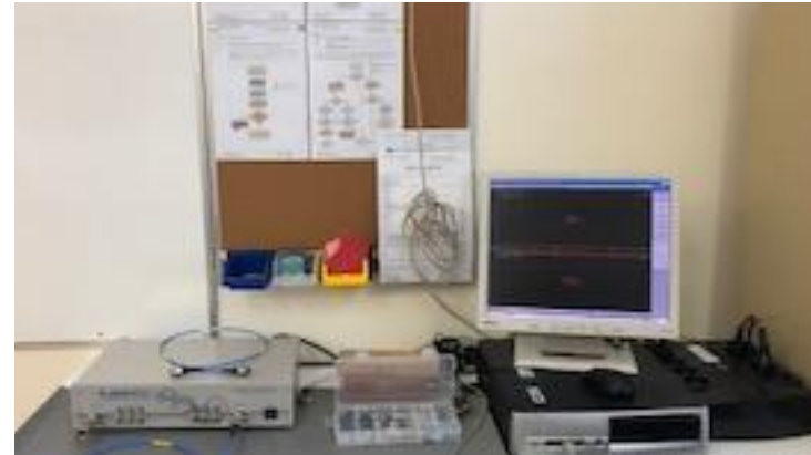
RF Cable Test Station + Copper Mountain Spectrum Analyser
