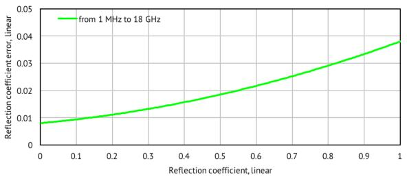
Specifications are based on isolating DUT ( $S_{21} = S_{12} = 0$ )
