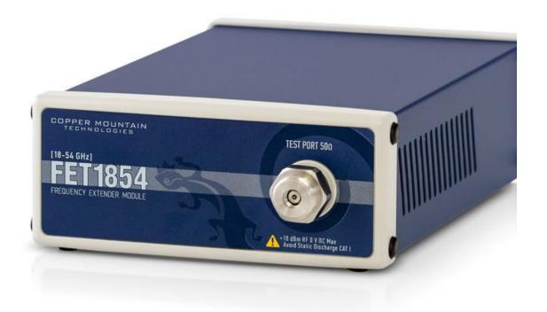
With the launch of the new FET1854 extenders, the CobaltFx system will allow engineers to build a scalable and affordable 5G testing solution. Anchored by a 2- or 4-port 9 or 20 GHz USB vector network analyzer, CobaltFx includes extenders in multiple frequency bands: 18 to 54 GHz, 50 to 75 GHz, 60 to 90 GHz and 75 to 110 GHz. Frequency extension is a standard software feature.
