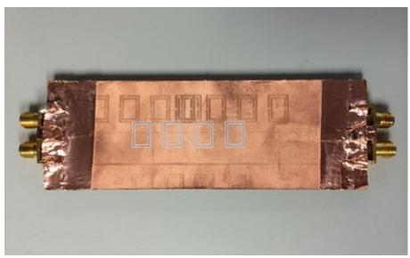
Figure 4 - Experimental common-mode Filter using split ring resonators designed by student Sang Goo under Dr. Ed Wheeler at Rose-Hulman Institute of Technology.
