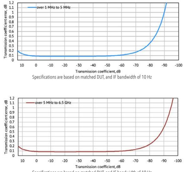
Specifications are based on matched DUT, and IF bandwidth of 10 Hz
