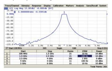
The VNA has a large frequency range with the option of frequency scan segmentation. This allows for optimal use of the instrument to realize maximum dynamic range while maintaining high
