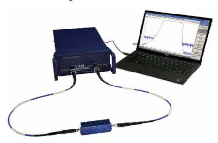
Cobalt VNAs have more than 162 dB dynamic range at 1 Hz IFBW, which allows them to maintain a wide measurement range at high measurement speeds. Measurement of all S-parameters of a BTS filter with full two-port and 801 measurement points with 1 MHz IFBW takes only 17.5ms while maintaining a measurement range of over 100 dB. This time is almost completely determined by the IFBW of the VNA. This measurement speed allows for real time tuning of high isolation BTS filters.
