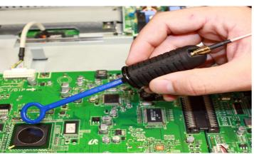
Pinpointing interference sources on a circuit board
